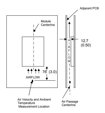
Wind Tunnel Test Setup Figure
